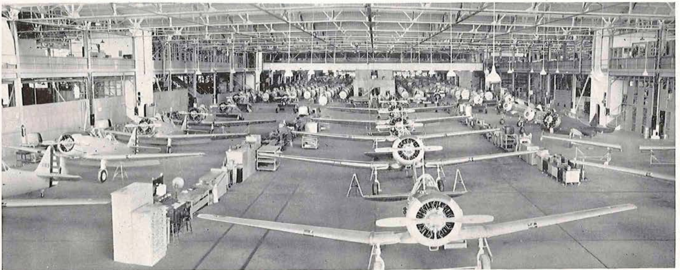
Straight-line production from fuselage frame to assembled airplane is evident in this view of North American's trainer assembly floor from the flight ramp. In the background ten fuselage assembly lines are discernible.
