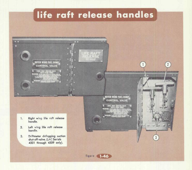
life raft release handles are shown on figure 1-46. In addition, provisions are made to stow one life raft in the galley coat closet and another in the aft right coat closet.
